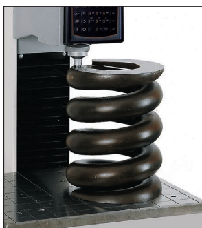
Clamping feature allows for testing large, overhanging parts with out the need for additional fixturing
